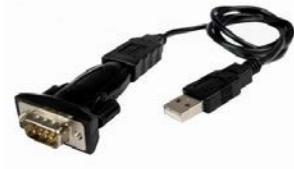
A black USB-to-Serial adapter cable with a standard USB A connector on one end and a DB-9 serial port connector on the other.                                                                                                                                                   |
