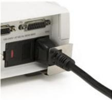
A white plastic power cord lock attached to the side of a white docking station, with a black power cord plugged into it.                                                      |
